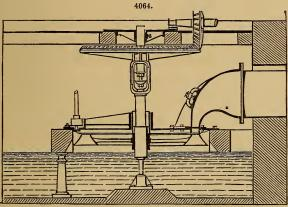
bottom of the central column or fixed spindle; for not-withstanding the employment of the hydraulic pivot, M. Girard, as a precautionary measure, employs the ordinary pivot suspended to the upper portion of the hollow spindle, as already explained.
